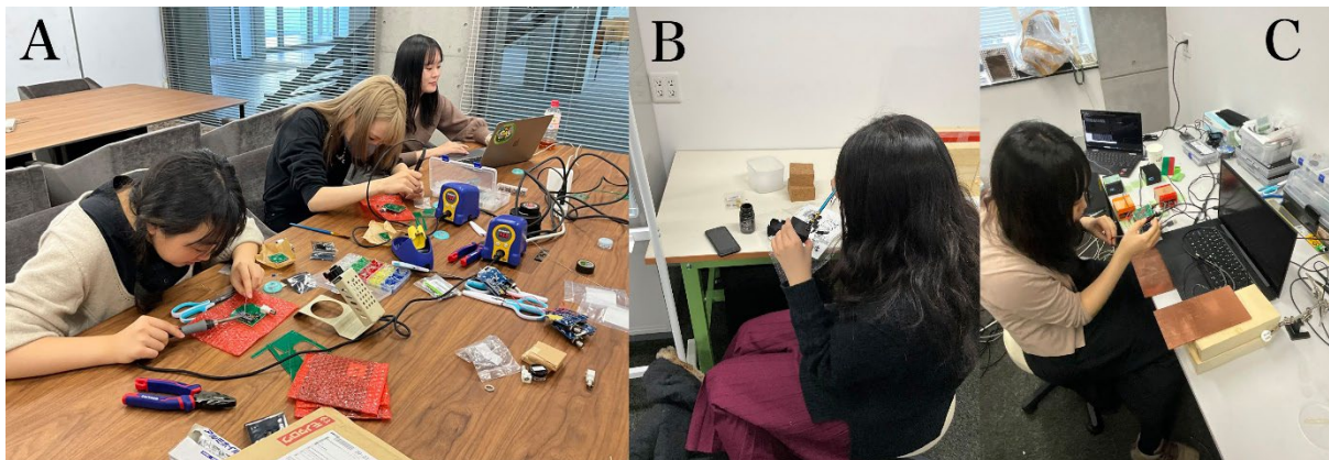
Fig. 1 Photos of developing the detector. A: Soldering the circuit board, B: Applying light-absorbing paint to the case for light shielding, C: Performance evaluation using a radiation source.
